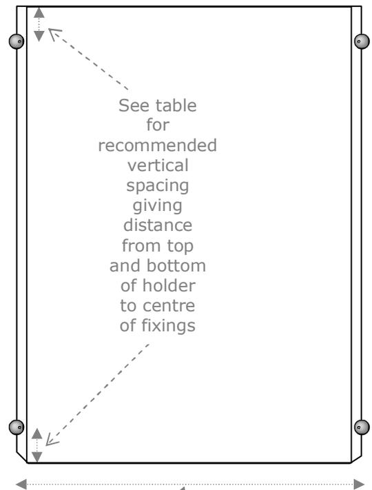
See table overleaf for measurement of horizontal spacing between centres of fixings, which is the same as the overall width of the poster holder, although we recommend adding 1-2mm to allow a small margin for error
