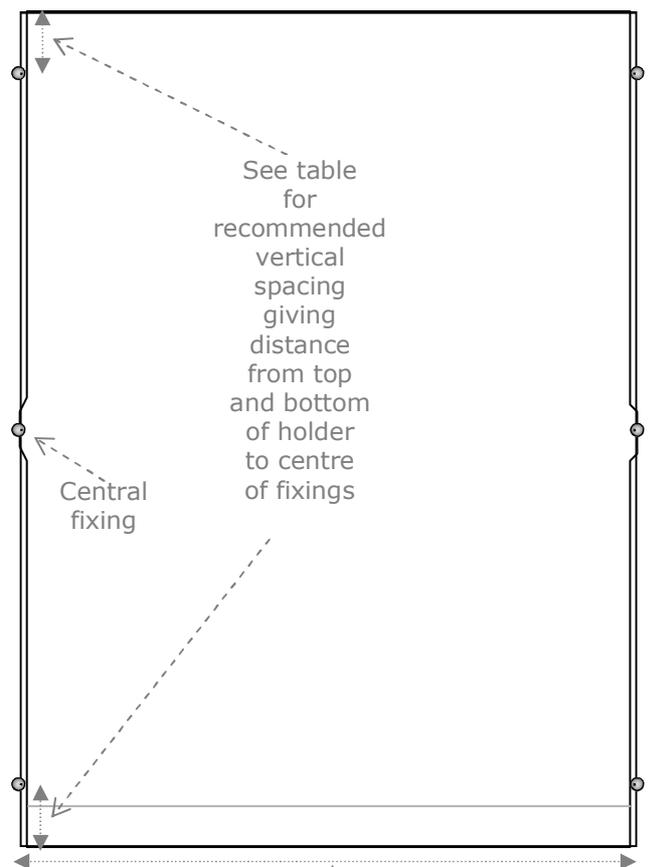
See table (page 2) for measurement of horizontal spacing between centres of fixings, which is the same as the overall width of the poster holder, although we recommend adding 1-2mm to allow a small margin for error
